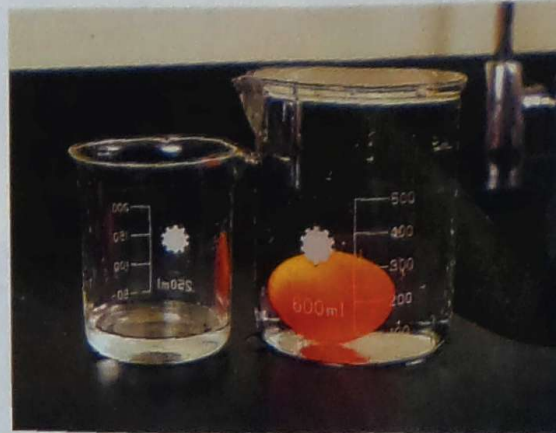
Figure 23 When the golf ball was dropped in the large beaker, it displaced some of the water, which was collected and placed into the smaller beaker.
